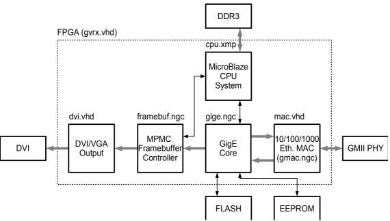
Figure 1: Block diagram of the receiver reference design
