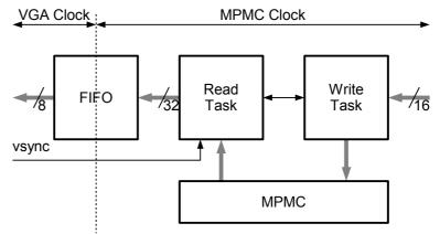
Figure 2: Block diagram of the framebuffer
